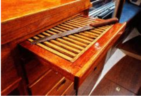
Detail work: a galley drawer is laid out for slicing bread. The crumbs collect under the grating.
