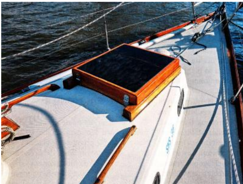
Improvement during refit: Hidden under the wooden frame is a watertight aluminium hatch.
