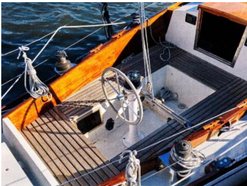
Angularity: Tiny wheel in small cockpit. The sharp corners and ergonomics originate from boatbuilding in wood.
